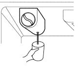
**NOTE** When filter is being removed, the water drains through the hole.
