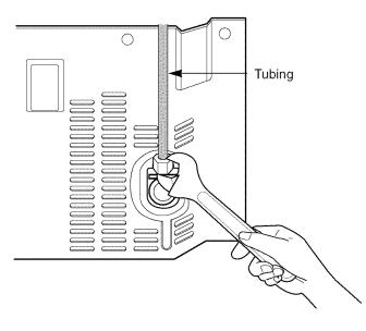
**A** CAUTION Check to see if leakage occurs at water line connections.
