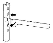
**A CAUTION** Make sure that shelves are level from one side to the other. Failure to do so may result in the shelf falling or spilling food.
