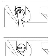
**3.** Flushing the Water System After Replacing Filter Dispense water through the water dispenser for 3 minutes to purge the system.
