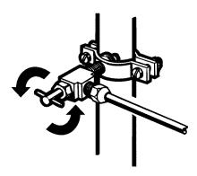
**2.** Insert the tube into the valve and fasten with wrench as shown in the figure below.
