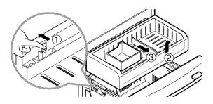
To install, after pulling out both rails as much as possible, and gently push down both left and right side while checking the hook on the front part.
