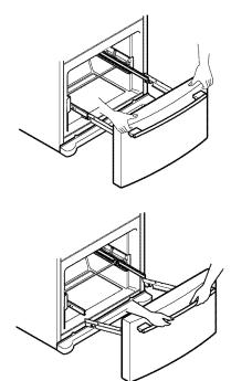
• With both hands, hold the center bar and push it in to let both rails fitted simultaneously.
