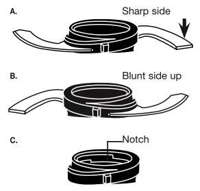
Pick up the blade ring by its hub holding ribs (grips) and line up the notches in the interior of the blade ring hub with the ridges on the sides of the plastic blade sheath. Let the blade ring slide down to the bottom of the plastic blade sheath. The lower blade should almost touch the bottom of the prep bowl.
