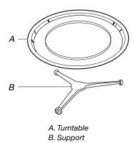
The turntable can rotate in either direction to help cook food more evenly. Do not operate the oven without having the turntable in place. See "Assistance or Service" to reorder any of the parts.
