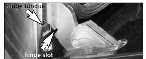
Fig. 6a Hinge assembly
