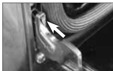
Fig. 25 Hinge retainer clip in locked position
