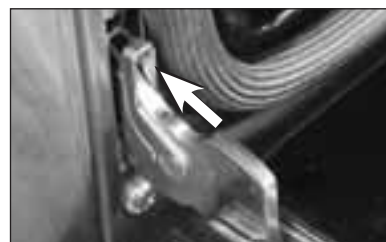
Fig. 25 Hinge retainer clip in locked position
