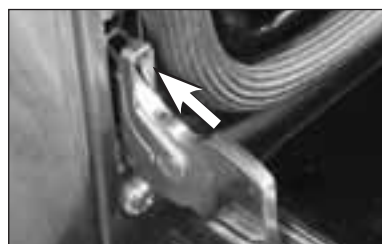
Fig. 25 Hinge retainer clip in locked position
