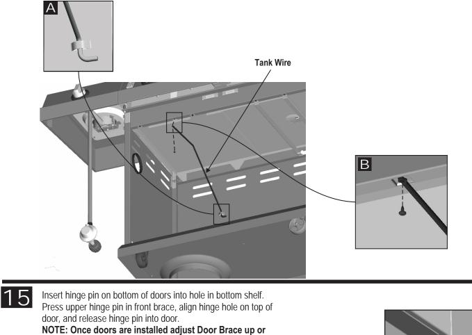
NOTE: Once doors are installed adjust Door Brace up or down to adjust for proper door clearance, then tighten screws to Door Brace from step 5.
