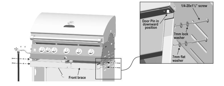
On back of grill, place upper back panel between side panels and above lower back panel. Secure upper back panel, in lower holes, using one 1/4-20x1<sup>1</sup>/<sub>2</sub>" screw, 7mm lock washer, and 7mm flat washer on each side. Do not fully tighten screws until side shelf installation is complete in later steps.
