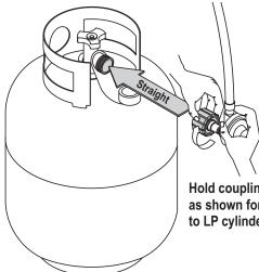
Hold coupling nut and regulator as shown for proper connection to LP cylinder valve.
