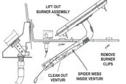
In some areas of the country, spiders or small insects have been known to create "flashback" problems. The spiders spin webs, build nests and lay eggs in the grill's venturi tube(s) obstructing the flow of gas to the burner. The backed-up gas can ignite in the venturi behind the control panel. This is known as a flashback and it can damage your grill and even cause injury.
