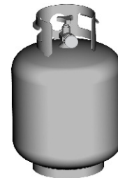
LP cylinder in upright position for vapor withdrawal
