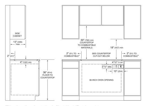
\*Minimum clearance from cooktop cut-out to combustible materials up to 18" (457) above countertop. NOTE: Electrical location applies only to installation with built-in oven.
