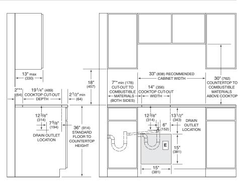
NOTE: Application shown allows for installation of two 15" (381) modules side-by-side with 33" (838) recommended cabinet width. 18" (457) recommended cabinet width for installation of single 15" (381) cooktop or module. "Minimum clearance from both side edges of cooktop cut-out to combustible materials up to 18" (457) above countertop. \*\*Minimum clearance from rear edge of cooktop cut-out to combustible materials up to 18" (457) above countertop.
