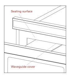
Waveguide cover location
