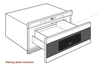
Rating plate: Open the drawer fully. The label is slightly beyond the back wall of the microwave cavity facing up from the flat surface.
