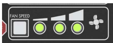
4 = HIGH (3 LED LIGHTS ON STEADY)
