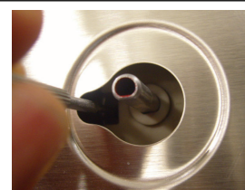
Adjustment screw next to the valve shaft
