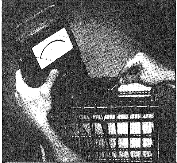
FIG. 34—USE AN OHMMETER TO CHECK THE ELECTRONIC CELLS FOR SHORT CIRCUITS.
