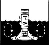
a continuous rollover action that provides a thorough cleaning of the wash load.
