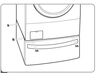
Make sure the holes on the pedestal align with the holes in the appliance, then install 4 screws at each corner to securely attach the appliance to the pedestal.
