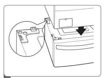
Make sure the back feet are in the correct positions.
