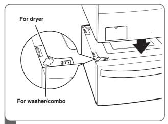
Place the dryer on the pedestal. Make sure the front and back feet are in the correct positions. The dryer feet will fi t into the innermost positions as shown.
