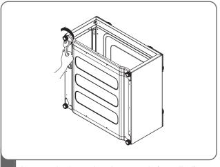
7 Loosen the leg using the wrench.(supplied)
