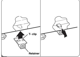
Insert the T-clip of the 4 retainers into the dryer base as shown. Press up on the back of the clip and pull outward to lock into place.
