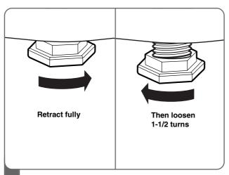
To set the dryer to the same height as the washer, fully retract the leveling feet of the dryer by turning them clockwise, then turn them counterclockwise 1-1/2 turns.
