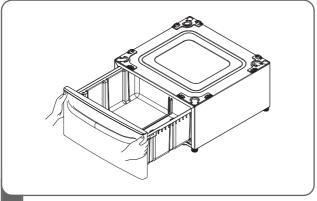
3 Pull up the drawer to disassemble.
