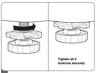
Make sure the leveling feet of the appliance are fully retracted.
