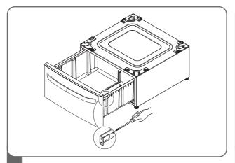
Remove two (2) screws on the either side of the drawer.
