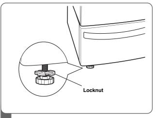
Securely tighten all locknuts by hand.
