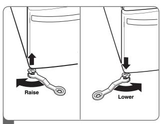
Loosen the locknuts on all 4 leveling feet of the **pedestal** until you can turn them with the wrench. Turn clockwise to raise or counterclockwise to lower until the pedestal is level and all 4 feet are solidly against the floor.
