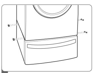
Make sure the holes on the pedestal align with the holes in the retainers, then install 2 screws at each corner to securely attach the appliance to the pedestal.
