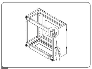
9 Remove four (4) screws (two on each side) on both side of slide.
