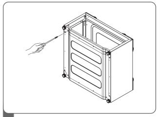
Remove twelve (12) screws on the bottom of the pedestal.
