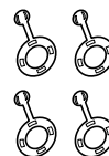
Cap (4 each) to cover the holes created after removing the shipping bolts
