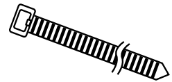
Tie strap to secure drain hose to standpipe, inlet hose, or laundry tub
