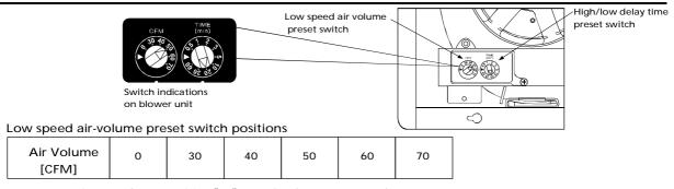
Factory setting: 50 CFM. Position"▶": Use for factory test only.
