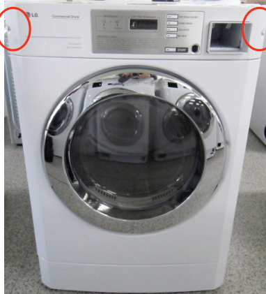
Disassemble the control plate
