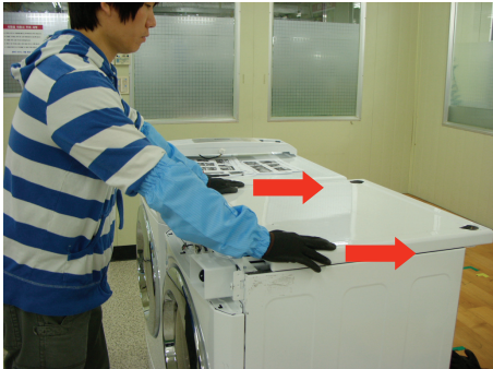
Disassemble the top plate
