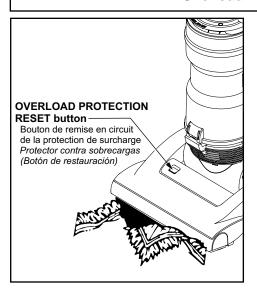
The OVERLOAD PROTECTION RESET button stops the nozzle motor when the brush jams to prevent belt breakage.
