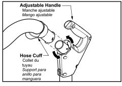
> To remove hose from adjustable handle; grasp hose by the hose cuff and rotate counter-clockwise, and slide off of handle.
