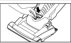
To replace the light bulb carefully insert securely into slot. Replace lens cover.
