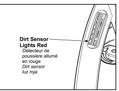
With heavy dirt concentration the dirt sensor is amber and red, indicating that POD power is at MAXIMUM. The vacuum cleaner operates at its highest energy consumption and noise levels.
