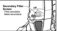
Every time dust bin is removed, rotate cleaning knob on top of dust bin until filter is clean to maintain cleaning performance.
