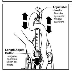
Press Handle Length Adjust button and raise handle to a comfortable operating position.
