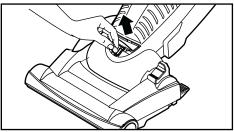
Remove the light bulb by pulling straight out.
