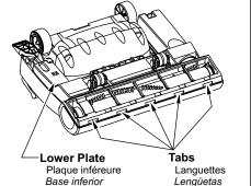
Reinstall lower plate. Ensure tabs are locked into slots.
