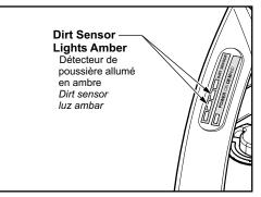
With normal dirt concentration the dirt sensor is amber, indicating that POD power is at HIGH. Energy consumption and noise levels increase.
