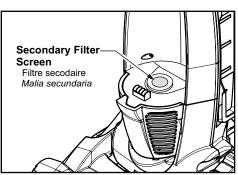
If the vacuum cleaner does not seem to have adequate suction, first check if the dust bin is full or if a filter is clogged.
