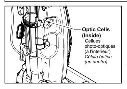
➤ The dirt sensor optics consist of two optic cells located inside the suction inlet. Occasionally, it may become necessary to clean the two optic cells to assure maximum performance.
