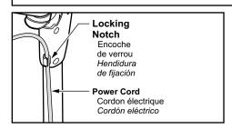
Make sure the power cord is placed into the locking notch as shown.
