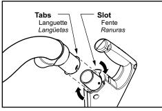
To reinstall hose to adjustable handle slide cuff onto handle and rotate clockwise to lock.
