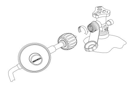
CAUTION! ASSEBLY TO PROPANE TANK. DO NOT USE TOOLS TO ATTACH REGULATOR / HOSE ASSEMBLY TO PROPANE TANK.
