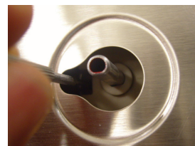
Adjustment screw next to the valve shaft
