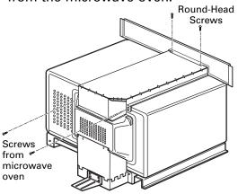
Place the top bracket on top of the upper duct, with the opening on the top bracket lined up with the opening on the duct. Attach the top bracket to the upper duct using two round-head screws.
