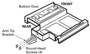
Install the rear duct to the bottom duct with one round-head screw.
