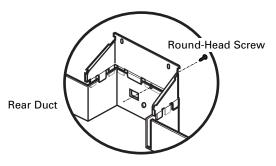
Remove all loose items, including the turntable and turntable support, from the microwave oven. Carefully turn the oven upside down. Remove one screw from microwave oven cabinet. Place the bottom duct assembly on the microwave oven bottom and fasten with six roundhead screws and the screw just removed from the microwave oven. Turn the microwave oven right side up, being careful not to bend the bottom duct flange.
