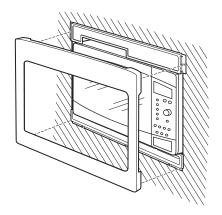
C Open the microwave oven door. Secure the trim frame using four flat-head screws (two on the inside top and two on the inside bottom).
