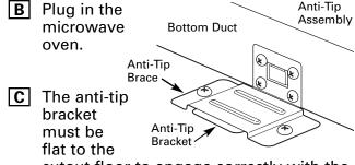
cutout floor to engage correctly with the anti-tip brace as shown. Carefully slide the microwave oven back, engaging the anti-tip brace. Make sure the power cord is not mashed or cut as you slide the microwave into place.
