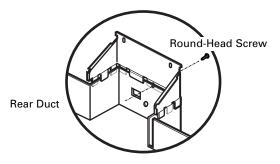
Remove a screw from right side (control side) of microwave oven cabinet. Place the bottom duct assembly on the microwave bottom and fasten with six round-head screws and the screw just removed from the side of the microwave. Turn the microwave oven right side up, being careful not to bend the bottom duct flange.
