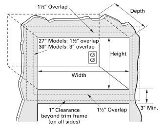
▲ WARNING — This trim kit uses air flow from the top, bottom and sides of the trim frame. Blocking the air flow can cause the microwave to function improperly and may cause damage to the microwave.
