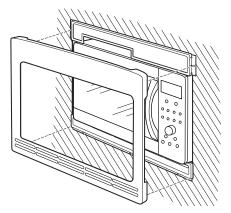
C Open the microwave oven door. Secure the trim frame using four flat-head screws (two on the inside top and two on the inside bottom).
