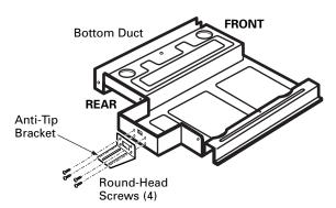
B Install the rear duct to the bottom duct with one round-head screw. Turn the microwave oven upside down.
