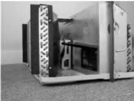
Figure 15 – Vent (Left side of unit)
