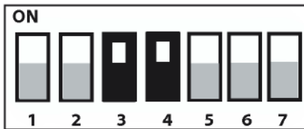
Figure 11 – Electronic Temperature Limiter Dip Switches
