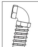
3. Tape the tubing pipe, drain hose and the connection cable. Be sure that the drain hose is located at the lowest side of the bundle. Locating at the upper side can cause overflow from the drain pan through the inside of the unit.
