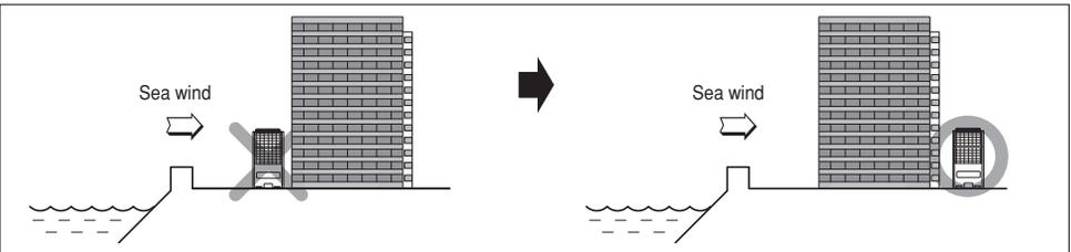
2) In case of installing the outdoor unit on the sea side, setup a windbreak to prevent sea wind.
