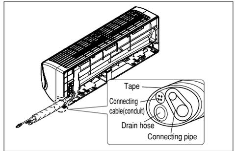
**Connecting the installation pipe and drain hose to the indoor unit.**
