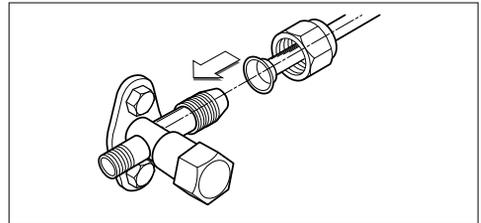
3. Finally, tighten the flare nut with torque wrench until the wrench clicks.
