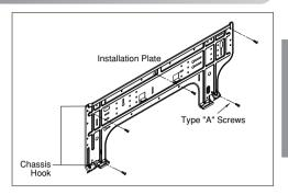
2. Measure the wall and mark the centerline. It is also important to use caution concerning the location of the installation plate. Routing of the wiring to power outlets is through the walls typically. Drilling the hole through the wall for piping connections must be done safely.
