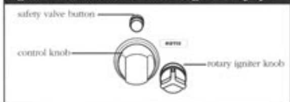
Figure 26-3 Rotisserie control, igniter, safety:
