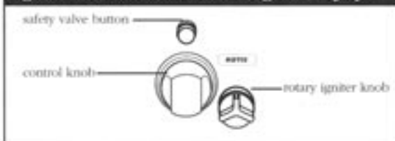
Figure 26-3 Rotisserie control, igniter, safety:
