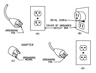
**WARNING**: This heater is for use on 120 volts. The cord has a plug as shown in A. An adapter as shown in C is available for connecting three-blade grounding-type plugs to two-slot receptacles. The grounding lug extending from the adapter must be connected to a permanent ground such as a properly grounded outlet box. The adapter should not be used if a three-slot grounded receptacle is available.
