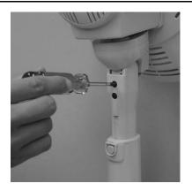
Insert and tighten the screws with a Philips screwdriver.
