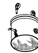
**1]** Carefully remove and set aside motor head and filter assembly
