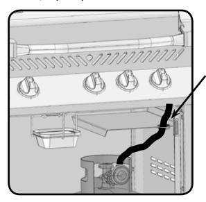
Ensure bushing snaps into propane heat shield as shown.
