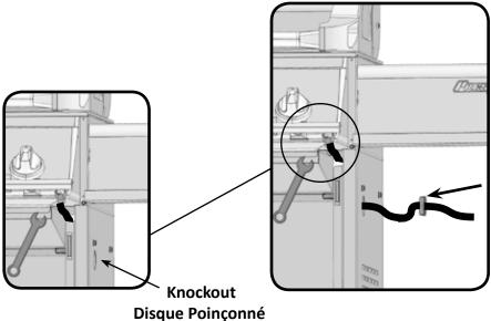
Ensure bushing snaps into side panel as shown.
