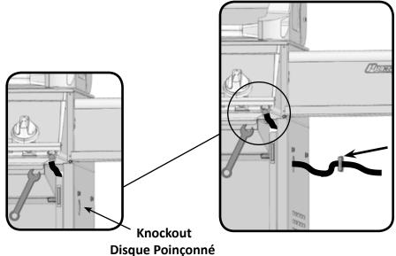
Ensure bushing snaps into side panel as shown.
