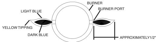
If the burner is getting too little air, the flames will be lazy yellow, and possibly produce soot. If the burner is getting too much air, the flames will be lifting erratically from the burner and may cause difficulties when lighting.
