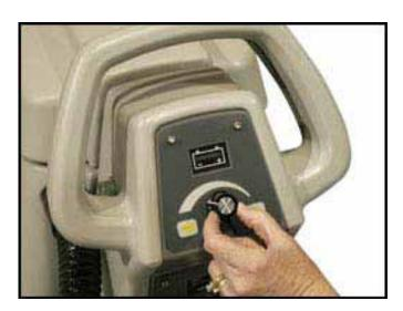
6. Turn the solution flow control dial to desired rate.
