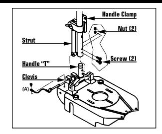
This burnishers is shipped without the handle attached to the chassis. Handle hardware kit (#372811) contains the necessary parts to attach the handle to the burnisher.
