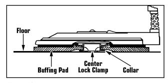
The floor pad packed with this burnisher **MUST BE** attached to pad driver before operating the unit.
