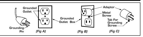
This floor machine is for use on a nominal 120 volt circuit, and has a grounding plug that looks like the plug illustrated in (Fig A). A temporary adaptor that looks like the adaptor illustrated in (Fig B & C) may be used to connect the plug to a 2-pole receptacle as shown in (Fig A) if a properly grounded outlet is not available.
