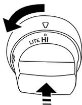
3. You will see the igniter glow. When burner is lit, release the knob. Turn knob to desired setting.
