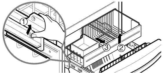
To install the drawer, pull out both rails to their full extension, raise the front of the drawer up and align the gears on the back of the drawer to rail assembly and gently push down on the front of the drawer until the tabs on each side snap into place.
