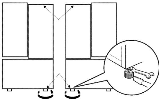
3. Open both doors again and check to make sure that they close easily. If not, tilt the refrigerator slightly more to the rear by turning both leveling legs clockwise. It may take several more turns, and you should turn both leveling legs the same amount.
