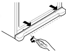
2. Turn the leveling leg clockwise to raise that side of the refrigerator or counterclockwise to lower it. It may take several turns of the leveling leg to adjust the tilt of the refrigerator.
