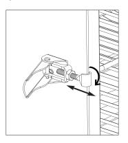
Loosen hex nut on door latch. Turn hook clockwise to tighten as shown. Secure hex nut firmly against door latch.
