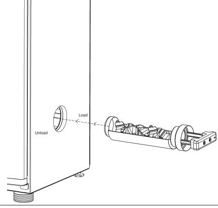
Before starting unit, place 1 cup of wood chips in chip loader. Never use more than 1 cup of wood chips at a time. Never use wood chunks.
