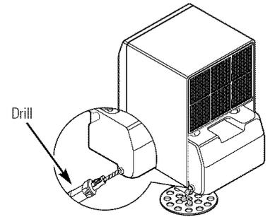
**NOTE:** The nozzle cannot be fixed after puncture. Use an ordinary garden hose cap (not included) to reclose if necessary.
