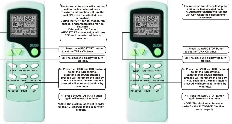
NOTE: The AUTOSTART and AUTOSTOP timers can be used in combination with each other.
