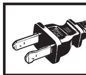
**CAUTION:** To reduce the risk of electric shock, **THIS PRODUCT HAS A POLARIZED PLUG** (one blade is wider than the other).
