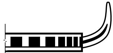
PROPER AIR SHUTTER SETTING
