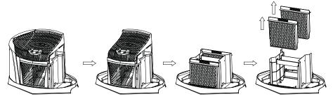
Figure A: 3D6 100 Assembly and Wick Placement
